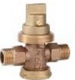
شیر کورب Curb Valve Model: KZ7782-100 Material: Bronze Size: 1/2-3/4 inch Max. W.P.: 10.5 bar
