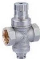
شیر کورب Curb Valve Model: KZ7782-100 Material: Bronze Size: 1/2-3/4 inch Max. W.P.: 10.5 bar
