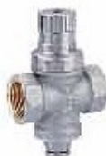
شیر فشار MINIPRESS Pressure Reducing Valve Model: KIZZPRV-015 Material: Brass Size: 1/2-3/4 inch Max W.P. inlet: 15 bar Max W.P. outlet: 4 bar
