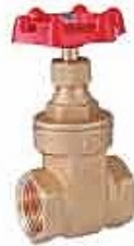
شیر گیت Gate Valve Model: KIZZV4-021 Material: Brass Size: 1/2-4 inch W.P.: 1/2-2 inch 16 bar 2 1/2-3 & 4 inch 20 bar
